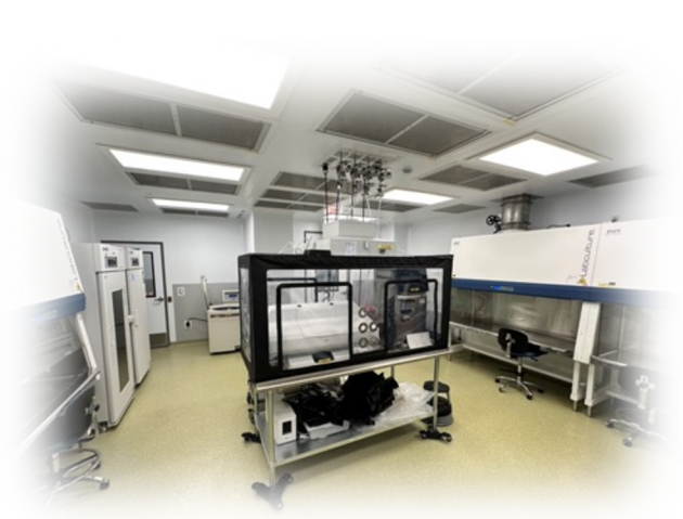
Biobubble with Wave bioreactor
